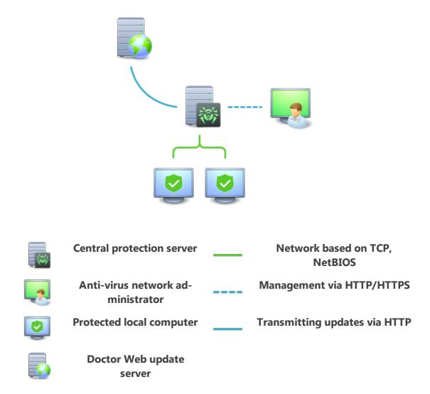
Figure 17. Logical structure of anti-virus network.
