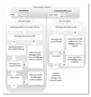
Scheme 1. Filtering messages in the transport system
